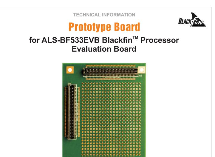
The Prototype Board is ideal solution for fast prototyping Customer specific application on base of ALS-BF533EVB Evaluation Board. This Prototype Board is equiped with ALS-BF533EVB compatible headers, large array of free pads and power supply paths.
