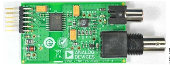
Figure 7. Photo of EVAL-CN0326-PMDZ Board
