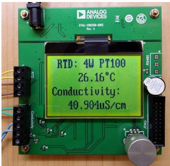
Figure 12. Photo of EVAL-CN0359-EB1Z Board Showing Home Screen in Measurement Mode
